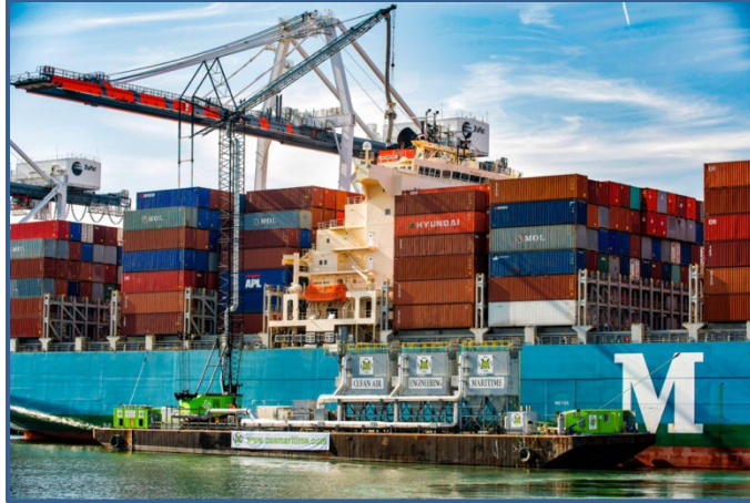
Figure 6: Barge-based capture and control system operating at the Port of Los Angeles (Source: Port of Los Angeles)
